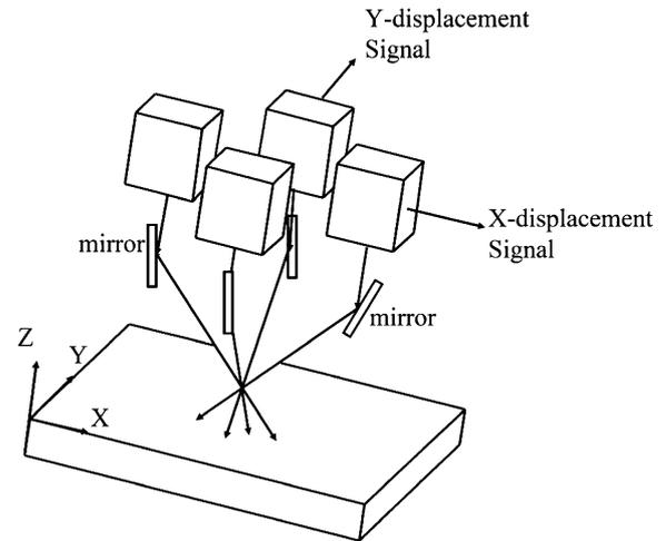
Fig. 9. Schematic of planar encoder.
