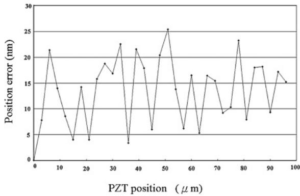
Fig. 8. Position errors between encoder and interferometer when stage moves through 100  $\mu\text{m}$ .
