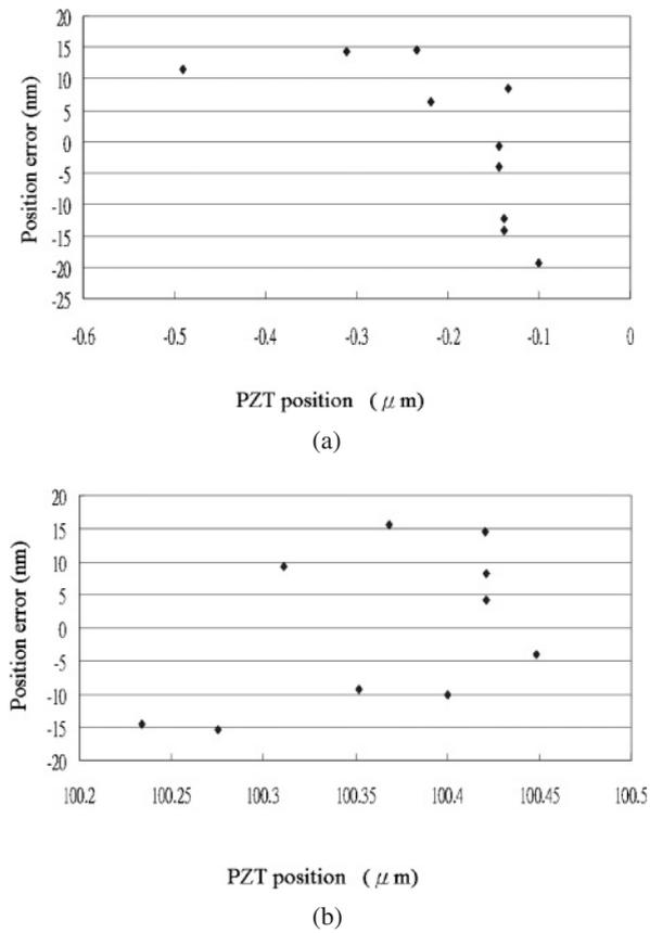
Fig. 7. The stage was programmed to move linearly back and forth 10 times through 100 μm. (a) Repeatability at starting point. (b) Repeatability at terminal point.
