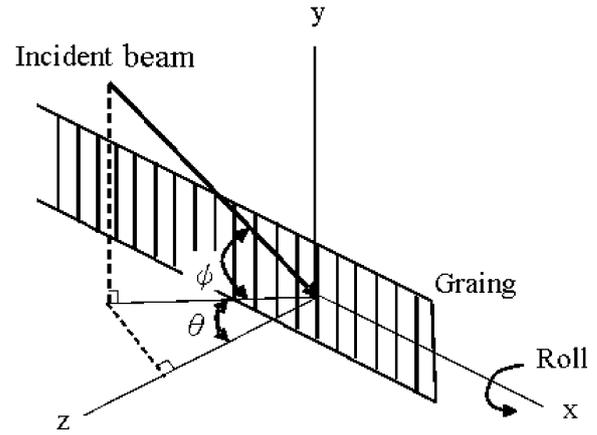
Fig. 4. Sketch of system during roll motion of grating. The fringe of the grating lies along the  $y$ -axis. The roll motion of the grating refers to a situation in which the incident light is not perpendicular to the  $y$ -axis.
