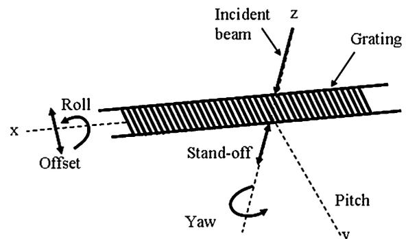
Fig. 2. Five degrees of freedom between grating scale and optical head.
