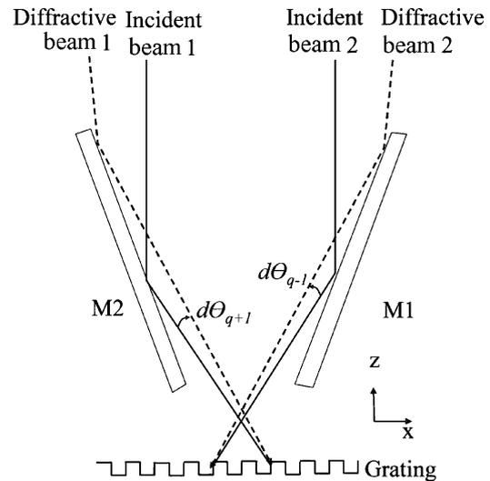
Fig. 5. Change in diffractive angle with roll motion of grating.
