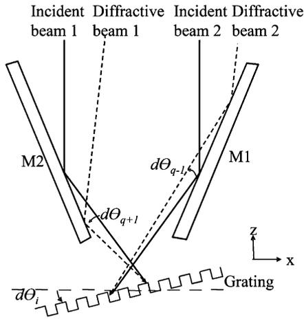
Fig. 3. Change in optical path with pitch of the grating.
