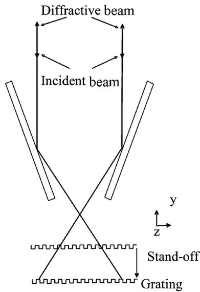
Fig. 6. Effect of change in gap. The gap does not affect the interference signal.
