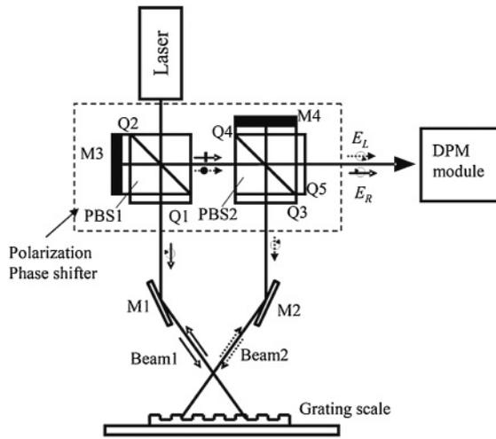
Fig. 1. Basic structure of proposed high-tolerance laser encoder.
